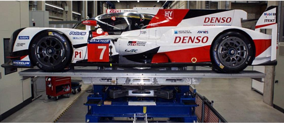
A specially-developed rig to determine, to a very precise level, the centre of gravity of a vehicle and the moment of inertia around the three main axes. Various complete cars can be mounted in exact road/track specification, up to a maximum weight of approximately 2,300kg.
